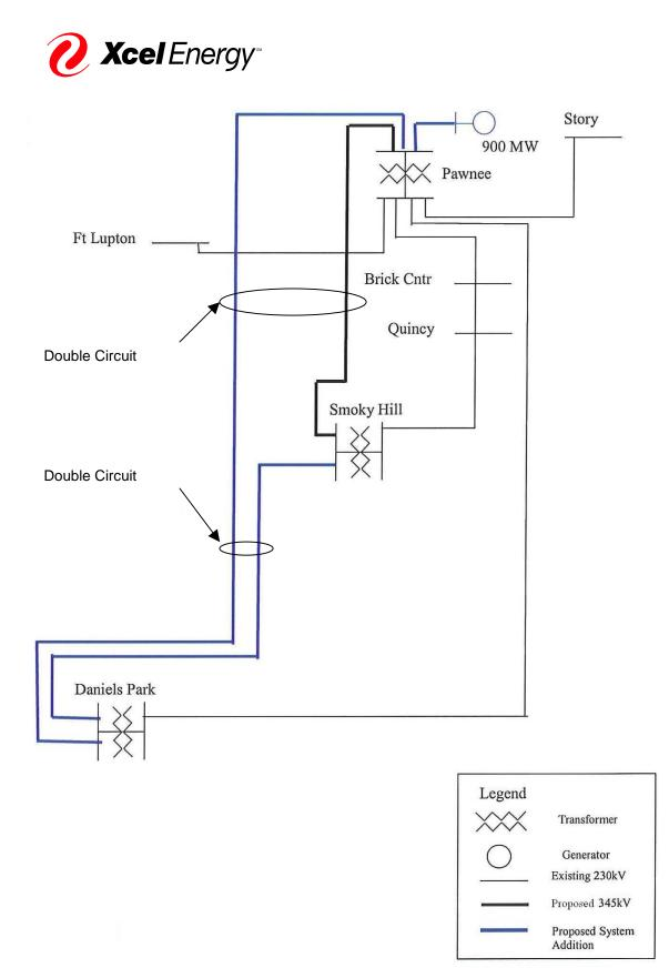
Figure 1: Proposed Pawnee One-Line Diagram (Upgrades Marked in Blue)
