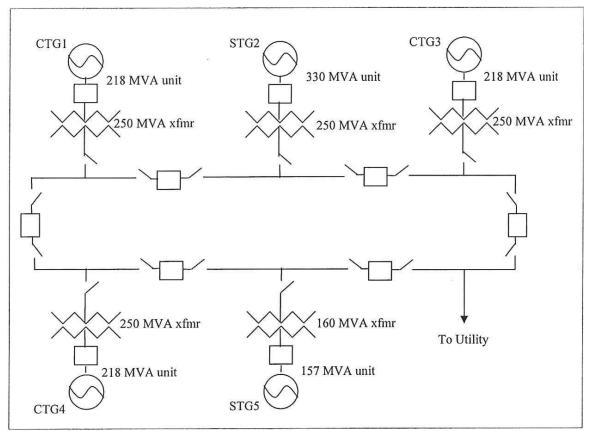
Figure 2: Proposed One-Line Diagram of Generator and Utility Interconnection
